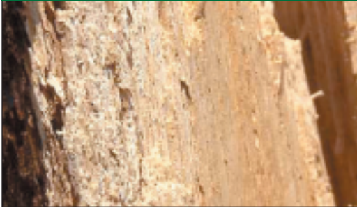
Photo 2a. White rot of an oak. White rot fungi decay the lignin and secondarily the cellulose components of wood. Significant strength loss in wood may develop only in the more advanced stages of decay.
