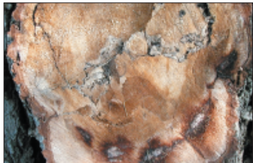
Photo 2f. Soft rot of a linden caused by Ustilina deusta . Soft rot decay causes a substantial loss in wood strength similar to brown rot.
