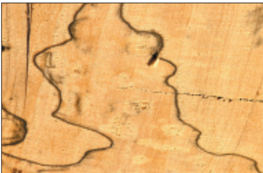
Photo 2e. Black zone lines formed by a wood decay fungus. Many different decay fungi form these zone lines as they decay wood. Therefore they are not diagnostic for any particular species.
