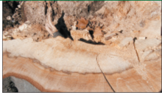
Photo 2b. White rot of a beech. White rot is considerably more common than brown rot.
