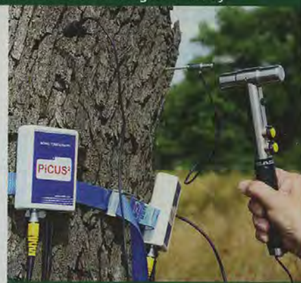
The PiCUS system uses a specialized hammer to induce sound waves through the tree, which are then detected by a series of sensors placed around the trunk.
