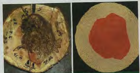
An output from a tree radar scan of the trunk cross section shows a stem with decay (left) and the predicted area of decay.
