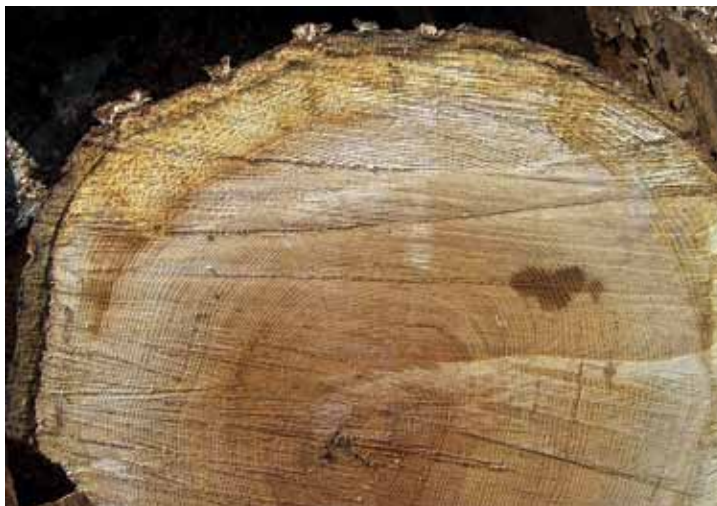
Figure 9. Sapwood decay cannot always be adequately quantified using sounding alone, although its presence may be identified.
