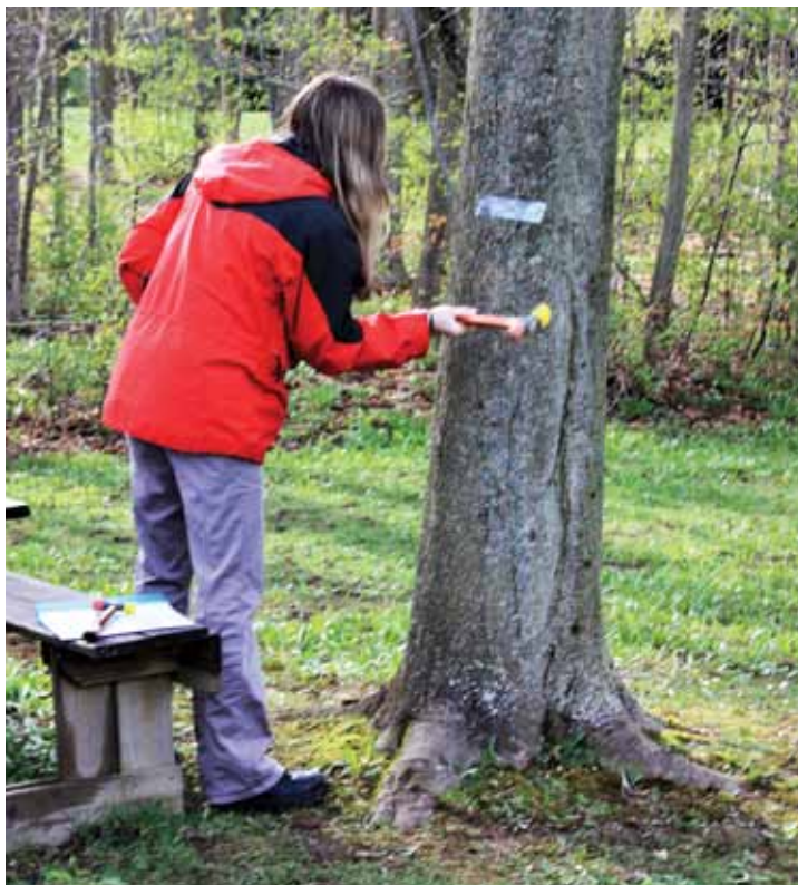
Figure 3. Sounding is a learned skill. It is best to establish a baseline resonance where the tree has solid wood and intact bark, from which tapping can assess the resonance, slowly moving toward the area in question.
