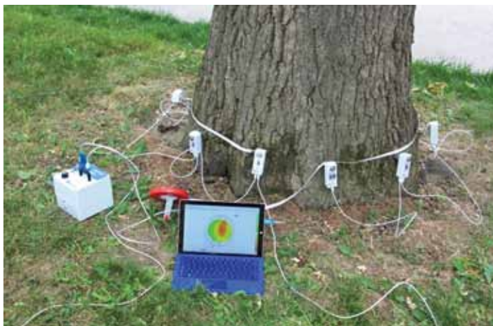
Figure 4. Sounding can be used to identify trees that may require advanced assessment techniques, such as tomography.
