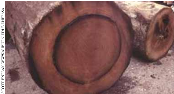
Figure 10. Ring shake can mimic an internal cavity in a tree. The resulting resonance sounds similar to that of a hollow created by decay.
