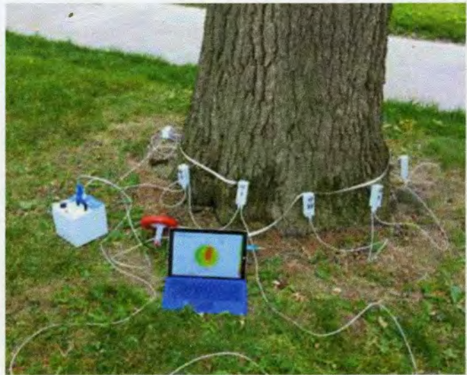
Figure 2. Sounding may identify the need for further advanced decay or risk assessment. A tomograph analysis was performed on this red oak ( Quercus rubra ) because sounding indicated the presence of significant internal decay.
