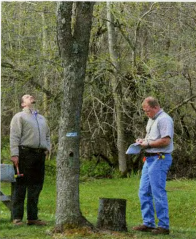
Figure 1. Sounding with a mallet or hammer can be part of a Level 2 or Basic tree risk assessment scope of work. Sounding also can be used in many other work contexts where structural assessment is valuable.
