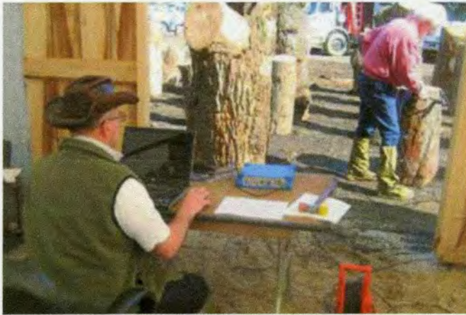
Figure 6. Accelerometer testing by Mucciardi et al. (2011) indicated that long duration, low-frequency wave forms were the best predictor of the presence of decay in a range of tree species. To the human ear this corresponds to a low, dull thud.
