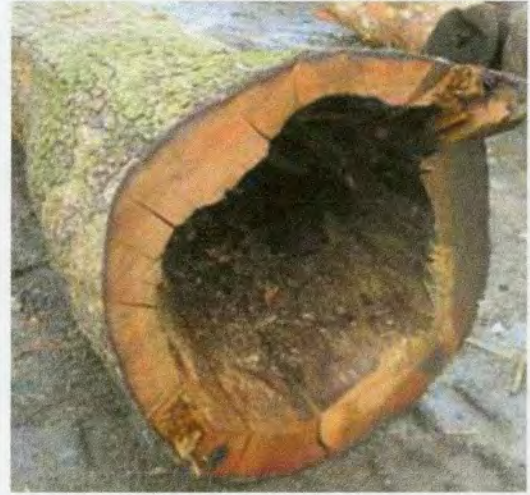
Figure 5. Psychoacoustic studies have shown that the human ear can detect subtle differences in resonance characteristics, once trained. Significant internal decay in trees, where cavities have left a thin shell of decayed wood, are a good starting point for training arborists on the use of sounding.
