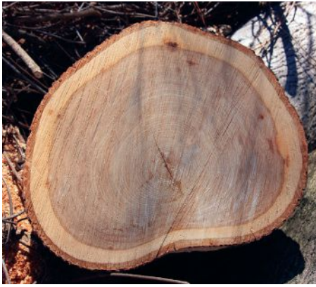
Photo 2: Heartwood in bitternut hickory. Many tree species form heartwood that may not show resistance to decay or may have only slightly increased resistance to decay.
