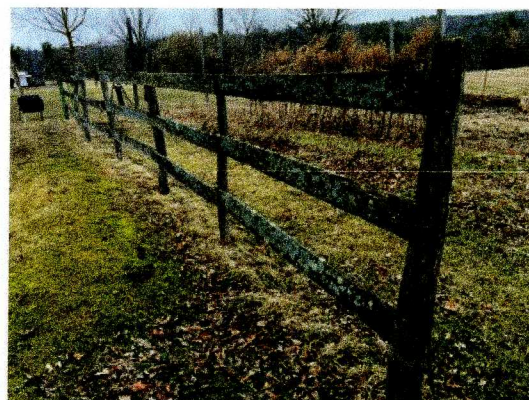
Figure 9. The elevated resistance of heartwood to decay in some tree species allows its use in service, as shown here for black locust fence posts and white oak rails. Photograph courtesy of Christopher Luley.
