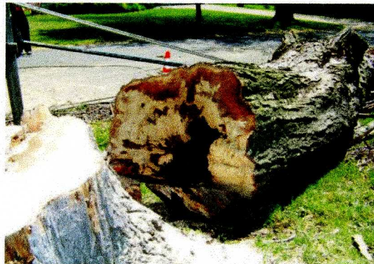
Figure 12. Knowledge of the wood types at the center of different tree species can impact safe tree care operations. Decay in the center of this sugar maple ( Acer saccharum ) resulted in failure of the hinge wood that was relied on for directional felling. Healthy, undecayed heartwood or sapwood are equivalent in most measures of wood strength. Photograph courtesy of Nate Wright, National Grid.
