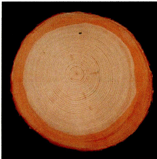
Figure 2. In a freshly cut and sanded disk of red spruce ( Picea rubens ), the sapwood is visible as an outer band of water-soaking. Upon drying, the sapwood becomes indistinguishable in appearance from the ripewood core. Photograph courtesy of Kenneth R. Dudzik, USDA Forest Service.
