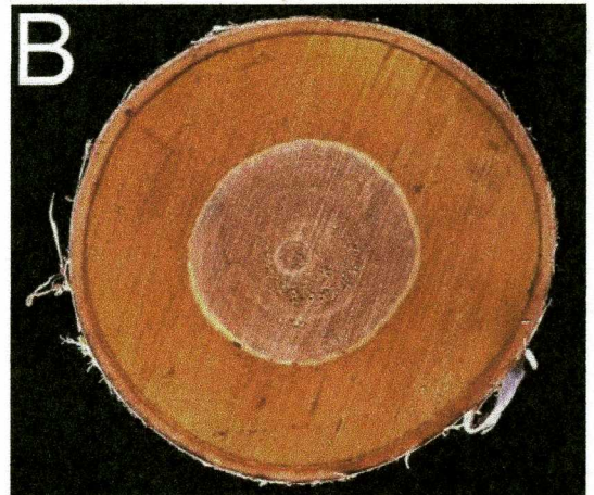
Figure 1. (A) Heartwood of pignut hickory ( Carya glabra ) surrounded by a thin band of lighter-colored sapwood. (B) Discolored wood from injury and infection in the core of paper birch ( Betula papyrifera ). Discolored wood is often misidentified as heartwood due to its central position in the stem and different or darker color. Photographs courtesy of Christopher Luley (A) and Kenneth R. Dudzik, USDA Forest Service (B).
